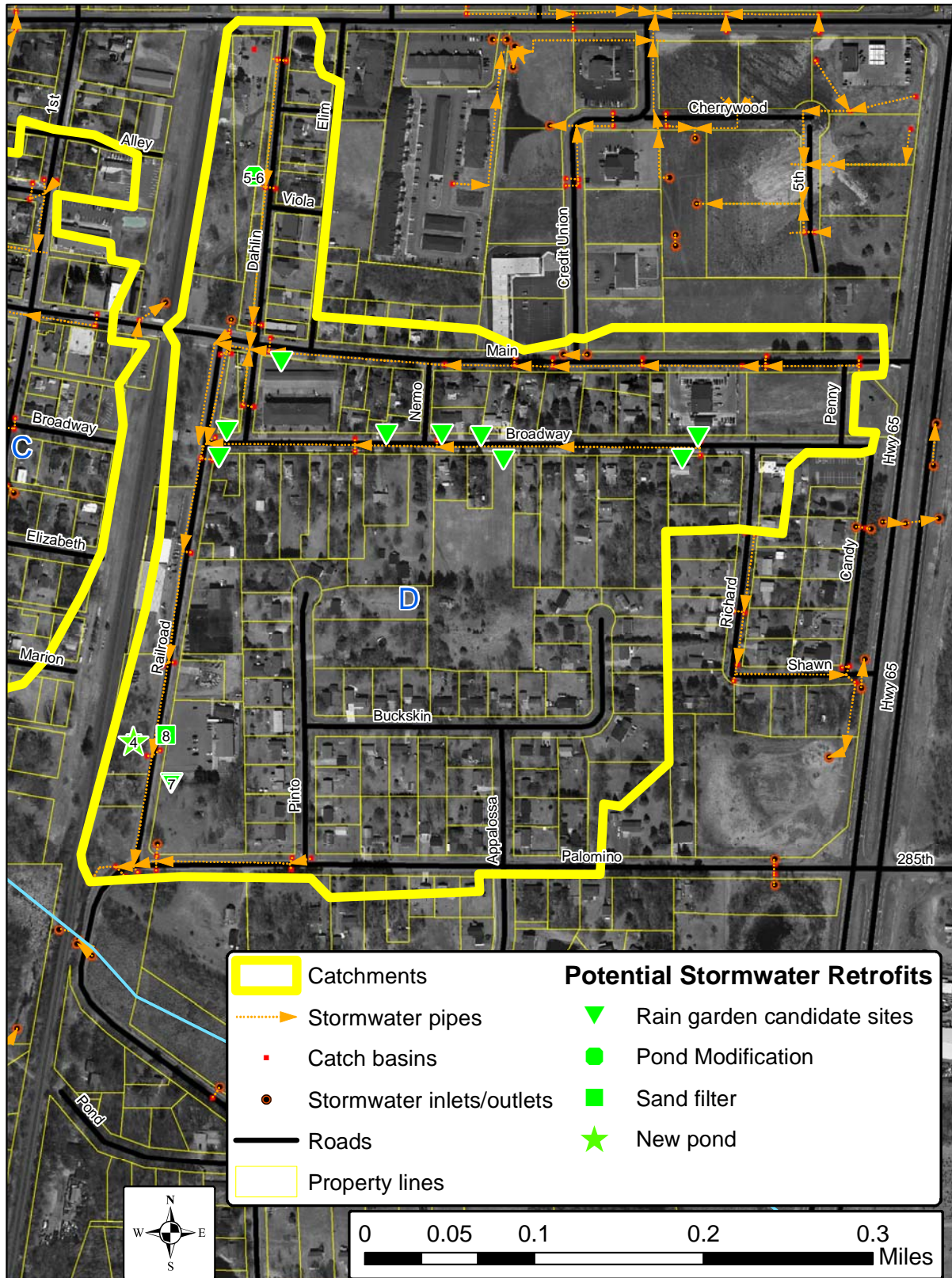
CATCHMENT D MAP AND RETROFIT RECOMMENDATIONS Retrofits, except candidate rain garden sites, are labeled with their project ID number (cost effectiveness rank).
