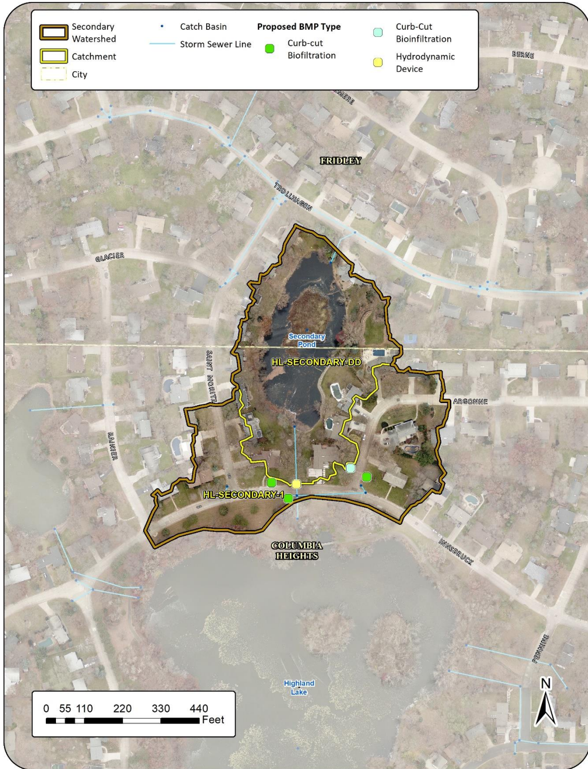
Figure 7: Study area map showing the proposed retrofits in the Secondary Pond drainage network included in this report.
