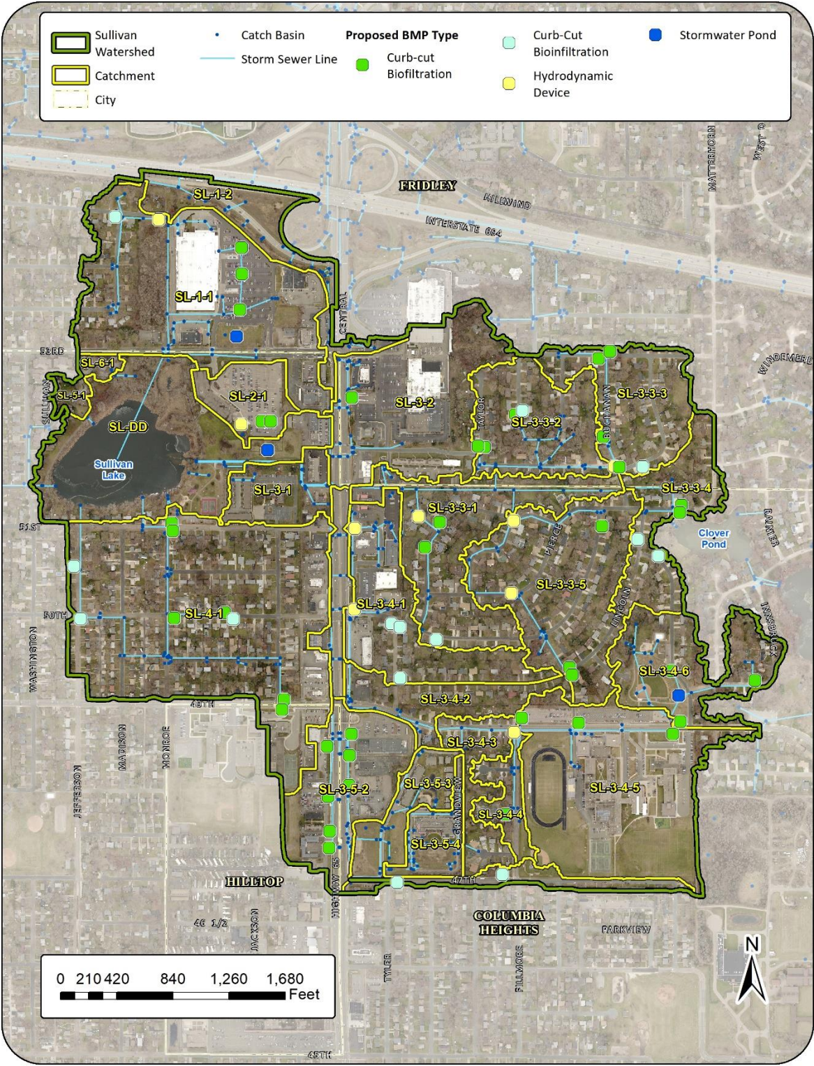
Figure 4: Study area map showing the proposed retrofits in the Sullivan Lake drainage network included in this report.
