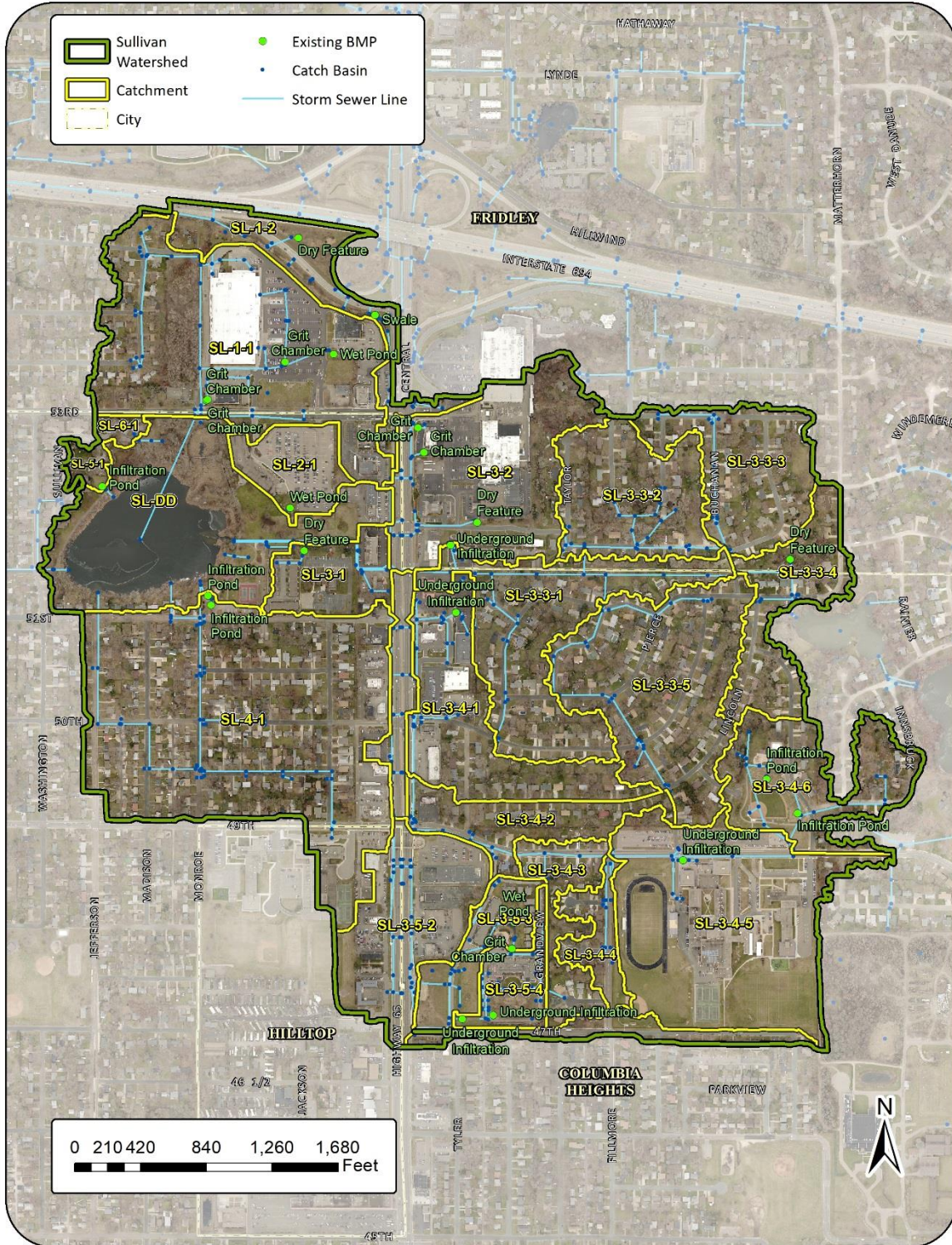
Figure 2: Sullivan Lake drainage network map showing existing BMPs included in the WinSLAMM model. Street sweeping is not shown on the map but was included throughout
