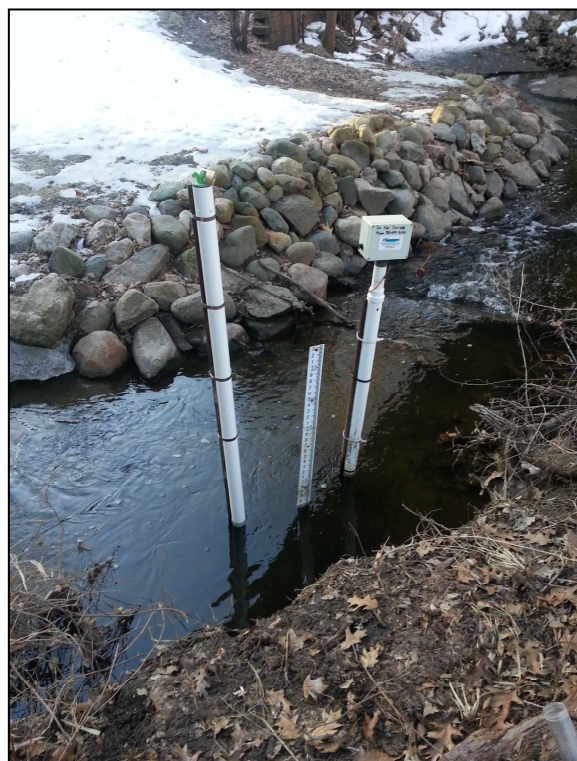
YSI EXO water quality sonde casing (taller) and an RDS continuous water level monitoring device in nearby Pleasure Creek. A staff gauge is shown in the middle.
