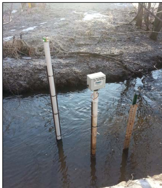
Hydrolab MS5 casing (taller) and a Measura continuous water level monitoring device I Springbrook Creek.
