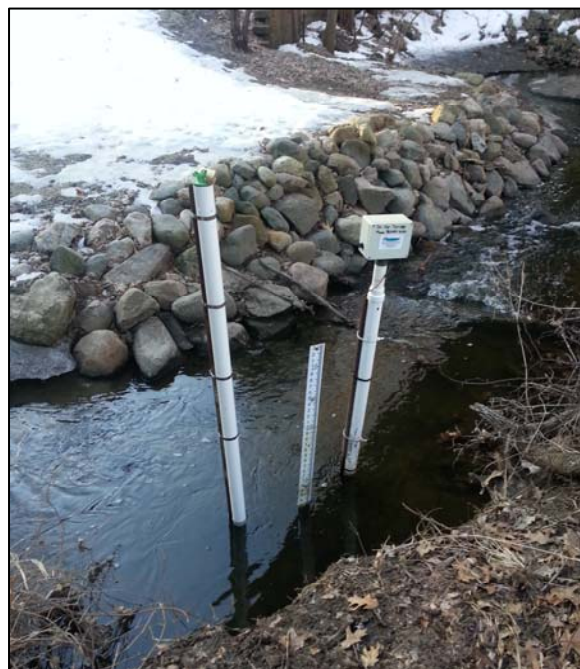
Hydrolab MS5 casing (taller) and a Measura continuous water level monitoring device in Pleasure Creek. A staff gauge is shown in the middle.
