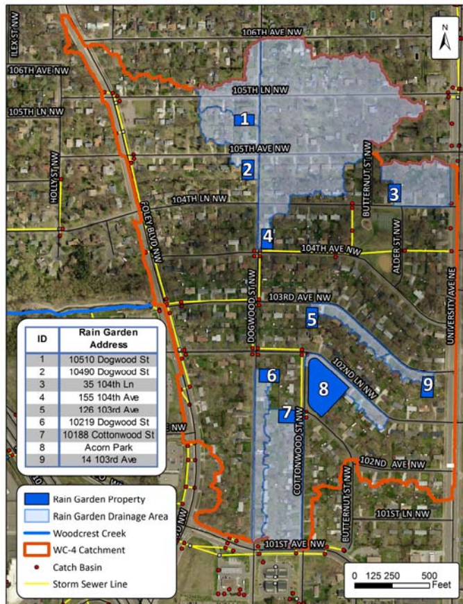
Sites of nine rain gardens installed in the WC-4 catchment of the Woodcrest Creek subwatershed in 2015.
