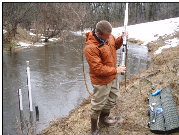
Staff deploying the Hydrolab MS5. In the background are the Hydrolab casing (shorter) and a Measura continuous water level monitoring device.
