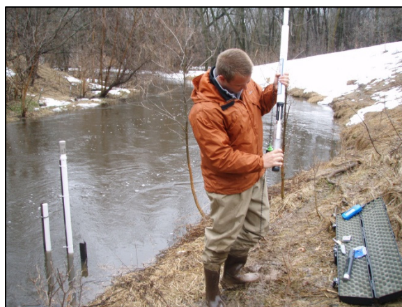
Staff deploying the Hydrolab MS5. In the background are the Hydrolab casing (shorter) and a Measura continuous water level monitoring device.
