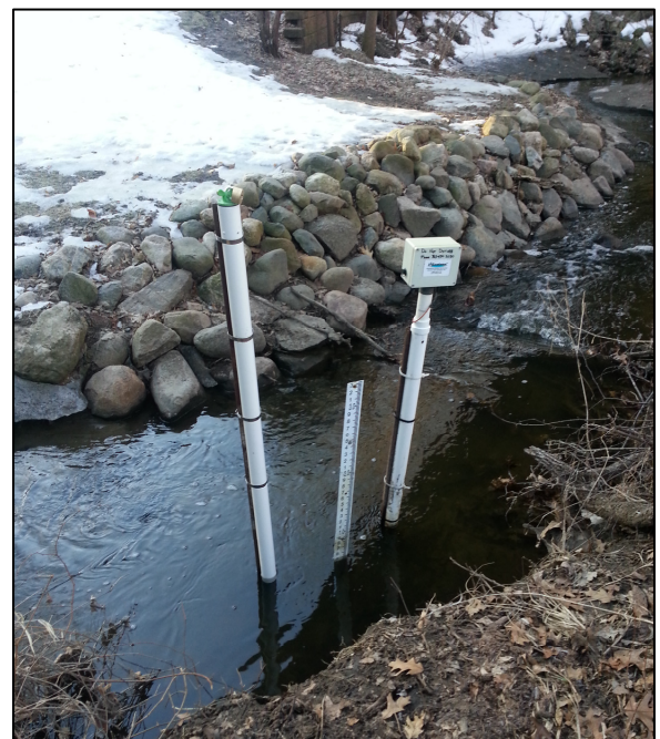
Hydrolab MS5 casing (taller) and a Measura continuous water level monitoring device in Pleasure Creek. A staff gauge is shown in the middle.
