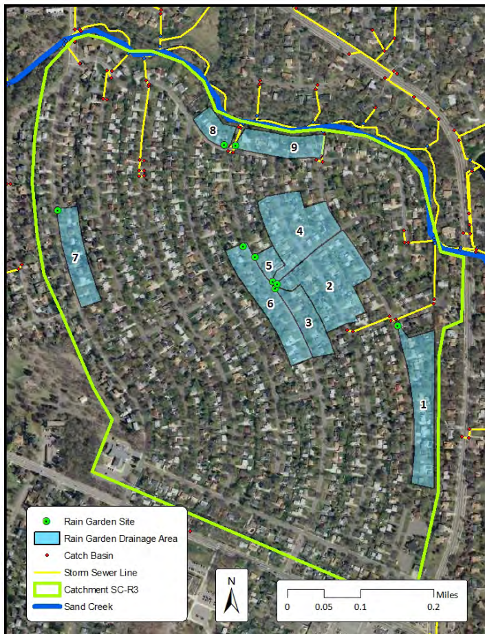
Installation sites of nine rain gardens installed in the Sand Creek subwatershed in 2012.
